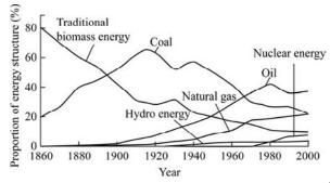
Figure 1 Changes in the world's energy resource structure since 1860<sup>1</sup>
