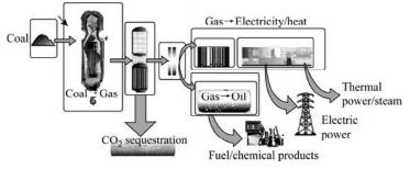
Figure 15 Schematic diagram of coal polygeneration [7]
