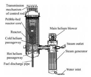
Figure 20 Schematic diagram of the primary-loop system in a high-temperature gas-cooled reactor<sup>29</sup>
