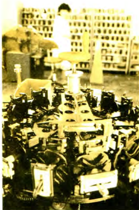
A 14-arm robot at the "Telemekhanika" plant in Nalchik gets radio components ready for installation.
