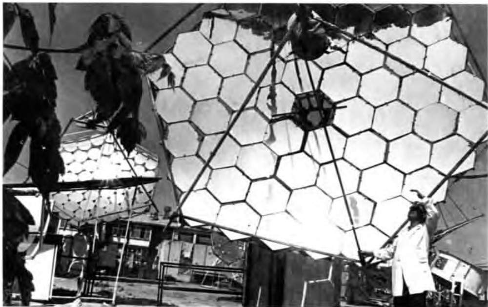
The future belongs to solar power engineering, especially in such a "sunny" republic as Uzbekistan. In the photo: concentrator mirrors at the testing ground of the Tashkent Institute of Physics and Technology.
