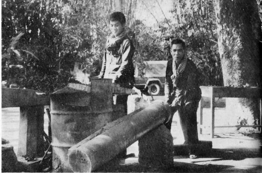
Workers of a farm tools plant made this bellows out of a captured weapon.
