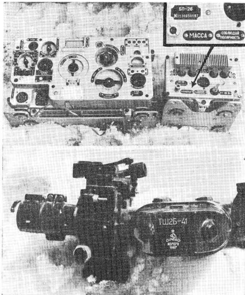
A radio transmitter-receiver ( upper photo ) and a telescopic sight ( lower photo ) from a tank of Soviet armed troops.
